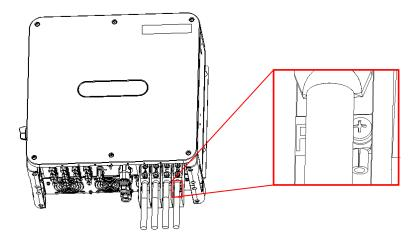
Figure 3-9 Ground connection terminal of AC side
