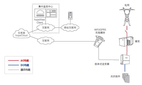
Figure 2-5 Distributed photovoltaic power plant networking design
