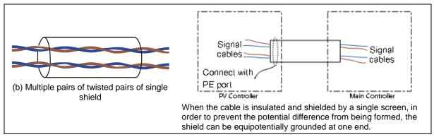
Figure 3-3 Twisted pair with shield
