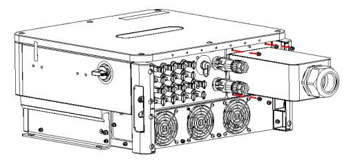
Figure 3-7 Disassemble the AC cable cover
