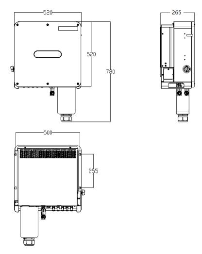
Figure 2-1 structural dimensions of hopeSun series (front, left, back, unit: mm)
