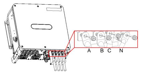
Figure 3-8 AC terminal block connection
