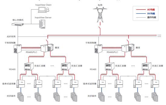
Figure 2-4 Large-scale ground photovoltaic power plant networking design
