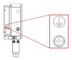
Figure 3-5 Protective grounding
