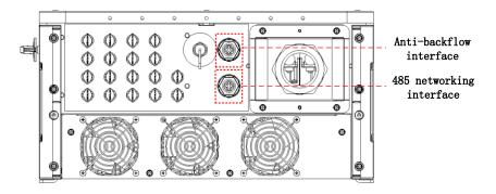
Figure 3-10 Location of RS485 and anti-backflow interfaces
