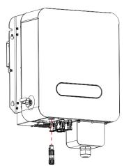
Lock the locking cap when the connection is complete. Check for gaps in the waterproof lock. If there is a gap in the waterproof lock, use a fireproof mud to block the gap.
