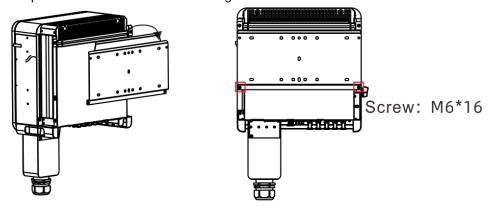
Figure 3-2 String inverter wall mounting diagram
