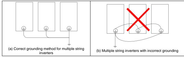
Figure 3-6 Multi-string inverter grounding
