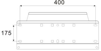
3. Fasten the fixing plate to the wall or bracket.
