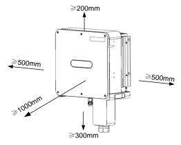
Figure 3-1 string inverter installation space
