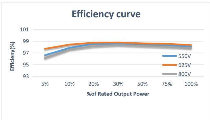
Figure 2-8 Power efficiency curve(take 80KW for example)
