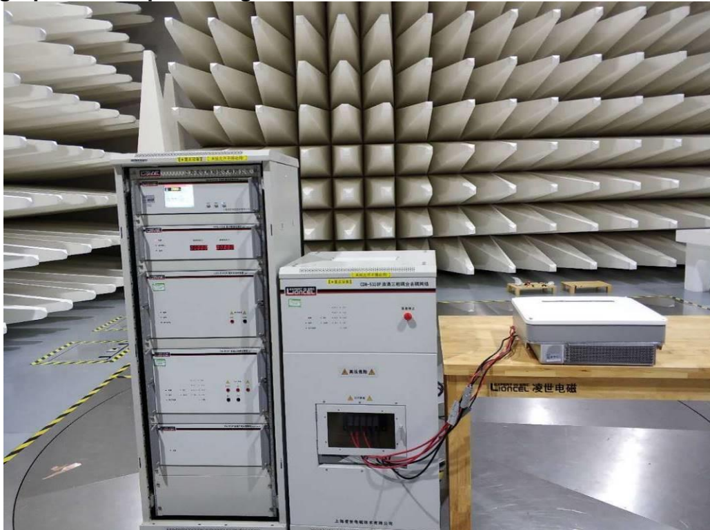
Photograph 8: Set-up for Surge
