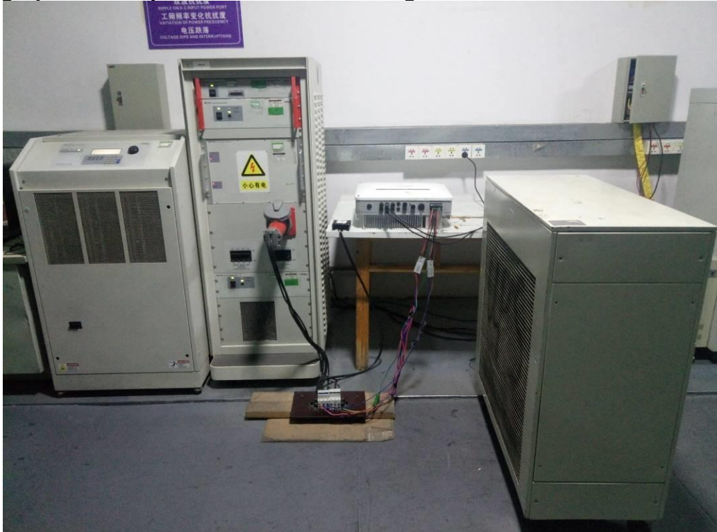
Photograph 1: Set-up for Harmonics & Voltage Fluctuations
