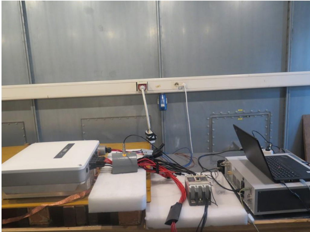
Photograph 6: Set-up for Power-frequency Magnetic Fields
