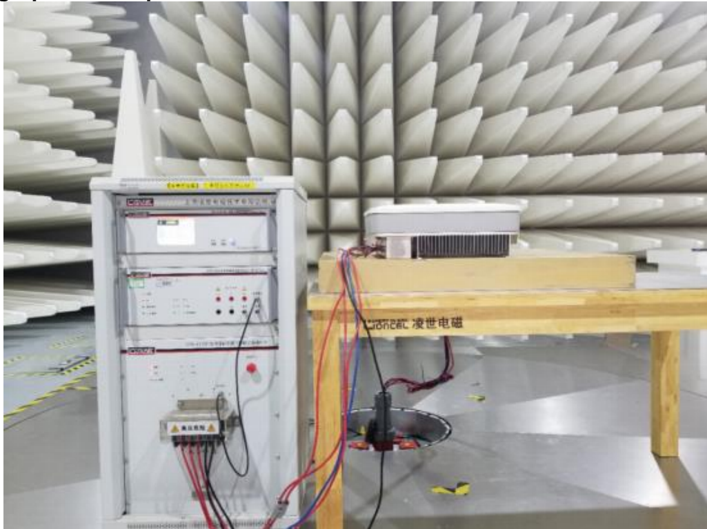
Photograph 7: Set-up for EFT
