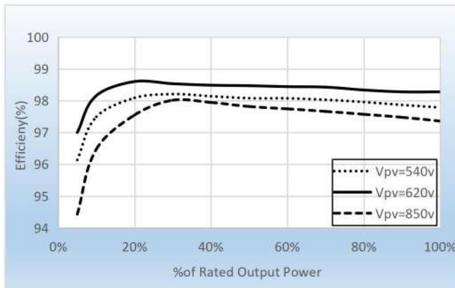
Figure 2-9 Power efficiency curve (take 50KW for example)
