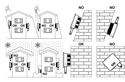
Figure 3-1Installation Position Selection
