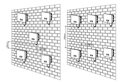
Figure 3-3 Clearance for multiple inverters
