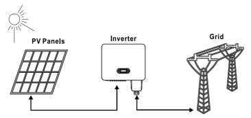
Figure 2-1PV Grid-Tied System
