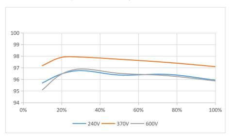
Figure 2-9 Power efficiency curve (take 25KW for example)
