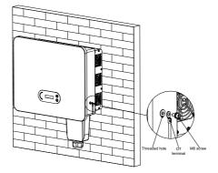
Figure 4-4 Inverter external grounding instruction diagram
