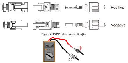
Figure 4-14 Use a multimeter to check the positive and negative electrodes
