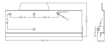
Figure 2-5 bracket dimensions (take 25KW for example)
