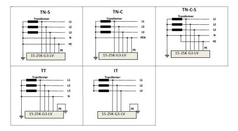
Figure 2-2 Overview of the grid configurations
