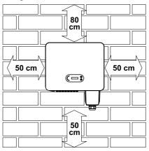
Figure 3-2Clearance for single inverter
