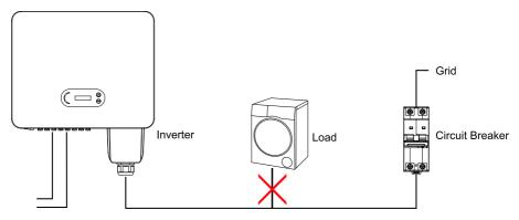
Figure 4-5 Incorrect connection between load and inverter
