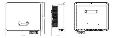
Figure 2-3 Front, side and back of the machine (take 25KW for example)
