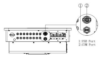
Figure 4-16 Communication connection Port
