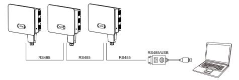
Figure 4-19 Multi SOFAR 15~25KTLX-G3-LV connecting Communications Register remote monitoring of SOFAR 15-25KTLX-G3-LV at its relevant website or APP according to monitoring device SN.
