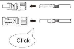
Figure 4-12 DC cable connection(3)
