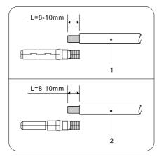
Figure 4-10 DC cable connection (1)
