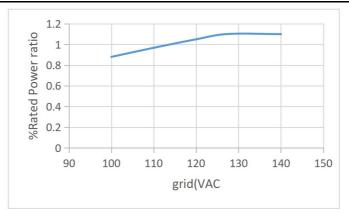
Figure 2-10 Rated Power ratio vs Grid Voltage
