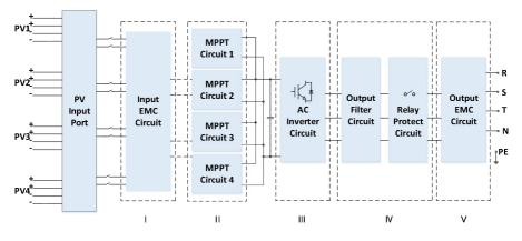
Figure 2-8 Schematic diagram(take 25KW for example)
